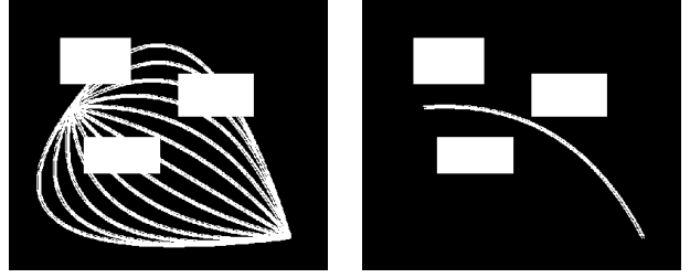
Figure 4: A set of polynomial paths (left figure) from start (upper left) to goal. The best path (right figure) is the shortest collision-free path in the set.
